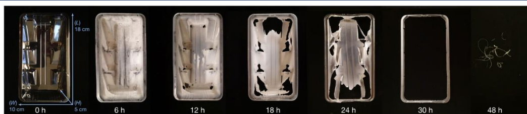
Figure 4. This picture shows FAST-PETase enzyme breaking down PET packaging product in 48 hours.
